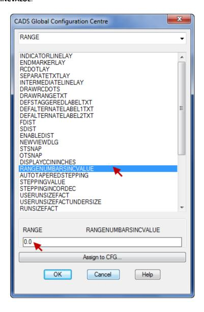
The default value is **0.0**. The value is a factor based on the spacing of bars. When the value is set to **0.5**, the number of bars are not incremented until the length of the range goes beyond **0.5 x Spacing**. For example, if the range length is 1000mm and the spacing is 100, there will be 11 no. of bars. When the value is set to 0.5, the number of bars will not be incremented until the length of the range exceeds 1050mm.
